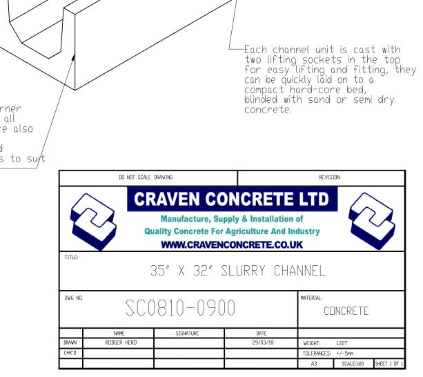
These robust precast reinforced concrete slurry
